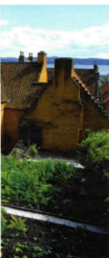
Crowstepped gables and pantiled roofs in the picturesque Fife town of Culross
